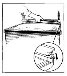
When drawers and covers are back in place, reinstall the gasket at the rear of the Sealed and Fresh drawer. Fit the end of the plastic drawer support into the slot on the gasket, with the rubber gasket flap facing you. Make sure the gasket snaps into place.
